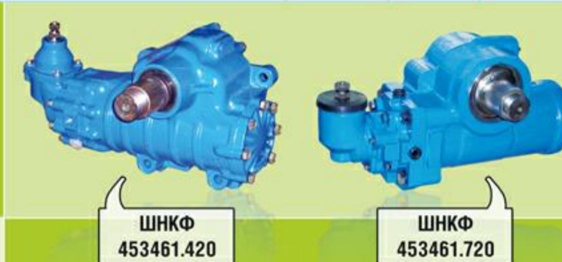
Construction of steering gears with hydraulic booster (integral type) consists of mechanical reducer, hydraulic distributor of rotary type, built-in booster jack. Emission type: screw → ball nut → piston-rack → bevel sector.
